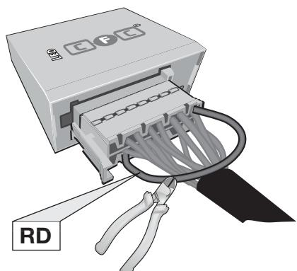
Pin 11 and Pin 2 disconnected
